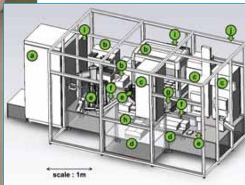
ADAM is a 5-meter-long robot whose equipment includes cameras, sensors, and computers in addition to (a) an automated -20°C freezer, (b) three liquid handlers, (c) three automated +30°C incubators, (d) two automated plate readers, (e) three robot arms, (f) two automated plate slides, (g) an
