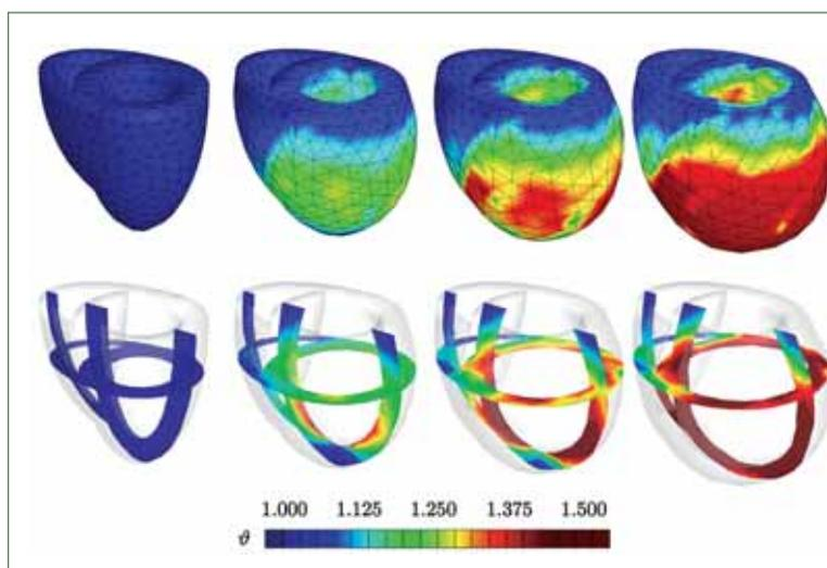
**An idealized ventricle discretized in space and time. After spatial discretization, the model consists of 4000 elements. In this simulation, the heart undergoes growth in response to volume overload—too much blood and therefore, too much stretch in the left heart chamber. The color map denotes the amount of growth. A value of 1 (dark blue) corresponds to the normal number of sarcomeres within the heart cell. A value of 1.5 (red) indicates a 1.5-fold increase of sarcomere units.**
